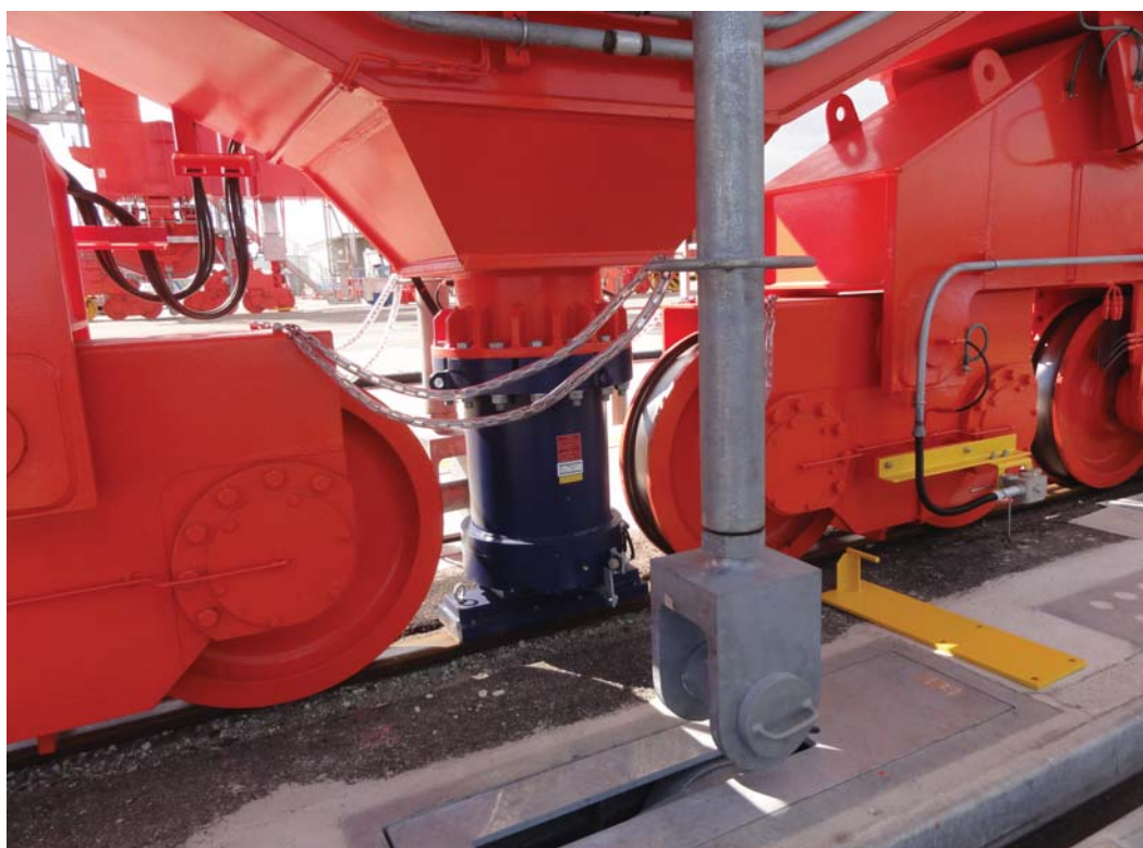
IRB-N mounted on container crane
