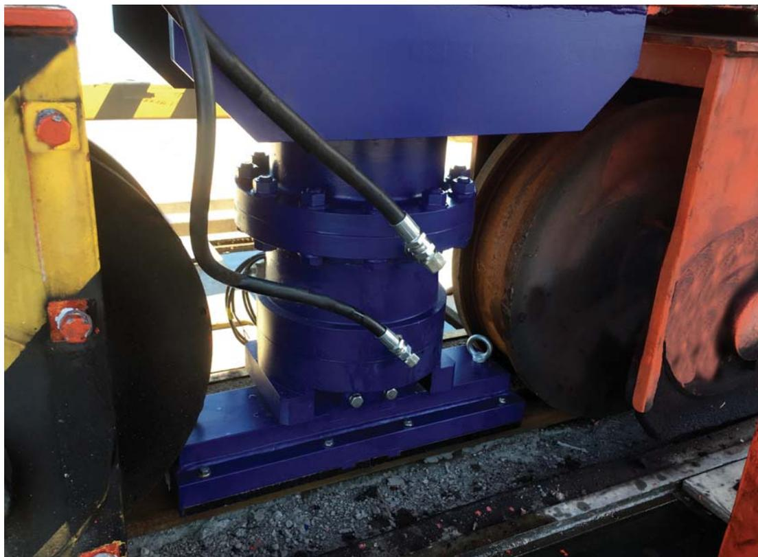
IRB-P mounted on container crane
