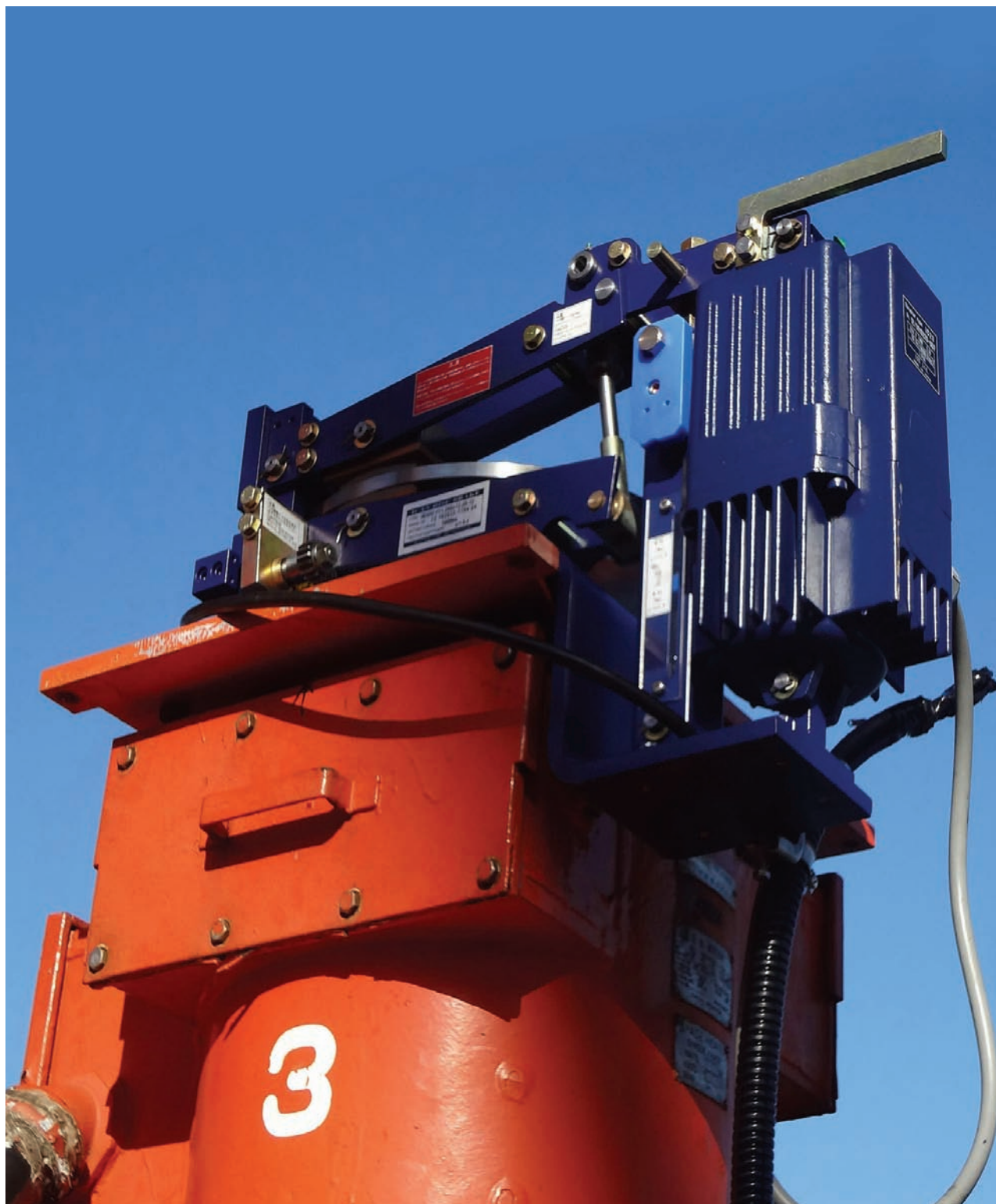
N-Mounted Brake (IB30V) on Container Crane at Surabaya, Indonesia
